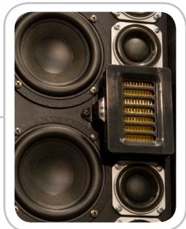
The LA880i uses eight 4.5-inch woofers, eight 2-inch midrange drivers and one 2.5-inch planar magnetics (ribbon) tweeter in an advanced design that provides a very short near-field extent and solid far-field performance.
